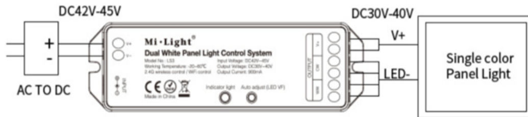
Single White Panel Light wiring diagram
